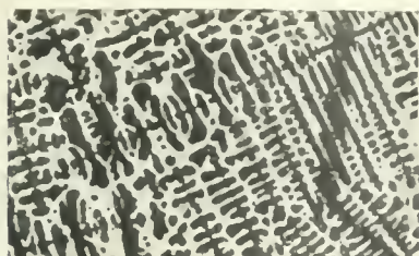
FIG. 4.—(Heycock & Neville, Phil. Trans. ) Copper-tin [tin 27.7%] chilled at 731° C. before complete solidification. Magnified 18 diameters. Blacks rich, whites less rich in copper.
